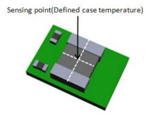
FIG 29. Case Temperature Sensing Point
