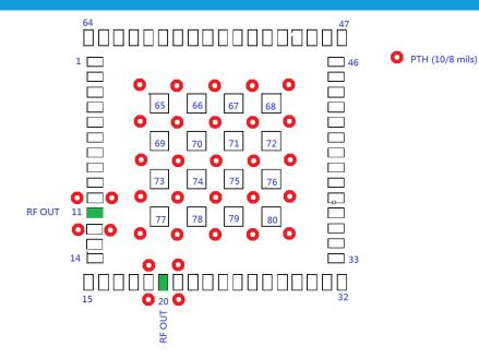
Recommend minimal via size and placement for grounding and thermal dissipation. Please double the ground via number when using laser via on HID process. More ground via and the use of 1-oz copper is recommended in our design to get better thermal dissipation.
