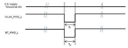
Figure 3: Wi-Fi and BT reset timing
