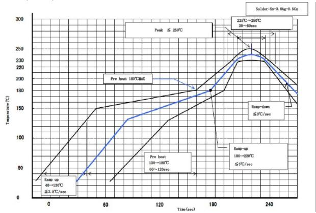
Ramp-up : 40 - 130 deg. Less than 2.5 deg./sec Pre heat : 130 - 180 deg. 60 - 120 sec , 180 deg. MAX Ramp-up : 180 - 220 deg. Less than 3 deg./sec Peak Temperature : MAX 250 deg.
