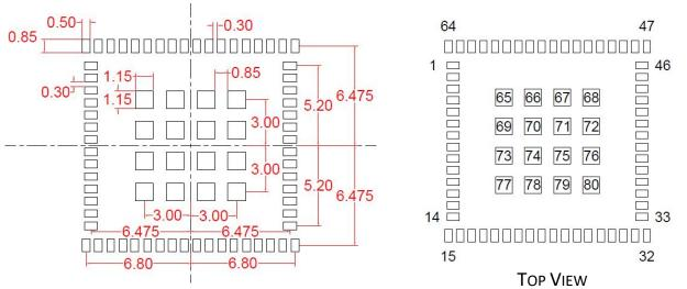
Figure 7: Pad dimensions and pin numbers
