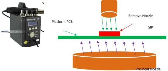
Remove the residue solder under the bottom side of SIP.
