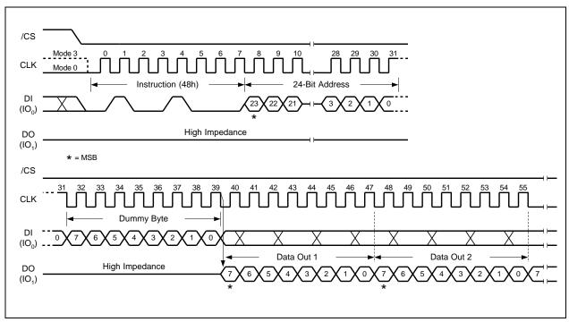
Figure 47. Read Security Registers Instruction (SPI Mode only)
