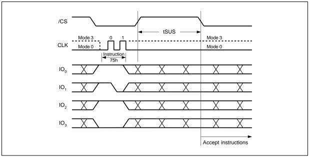
Figure 35b. Erase/Program Suspend Instruction (QPI Mode)
