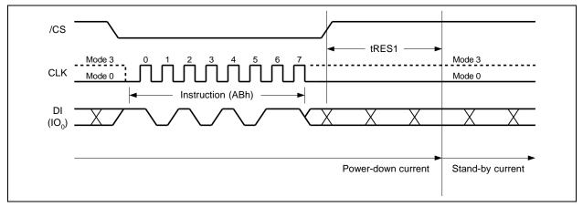
Figure 38a. Release Power-down Instruction (SPI Mode)
