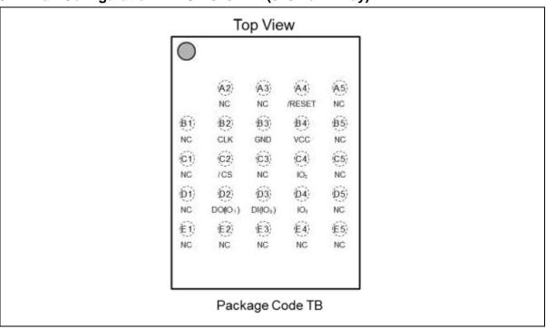
Figure 1d. W25Q64JW Ball Assignments, 24-ball TFBGA 8x6-mm (Package Code TB)
