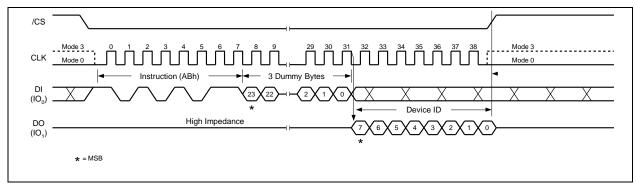
Figure 38c. Device ID Instruction (SPI Mode)
