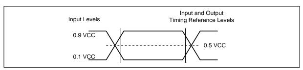
Figure 59. AC Measurement I/O Waveform
