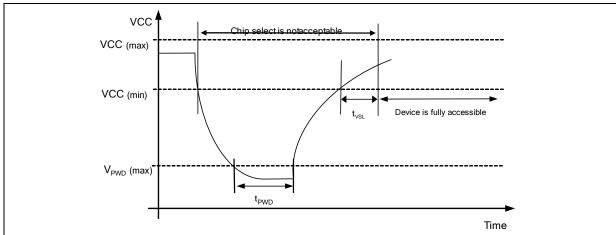
Figure 58c. Power Cycle Requirement
