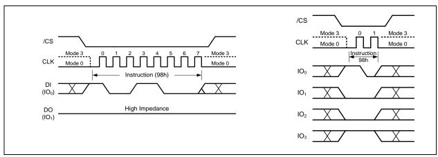
Figure 57. Global Block Unlock Instruction for SPI Mode (left) or QPI Mode (right)
