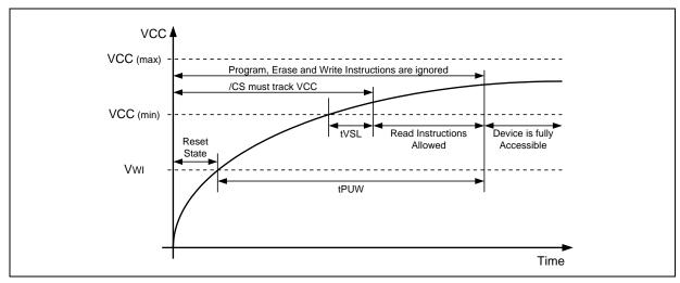
Figure 58a. Power-up Timing and Voltage Levels
