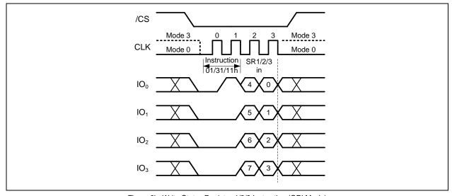
Figure 9b. Write Status Register-1/2/3 Instruction (QPI Mode)
