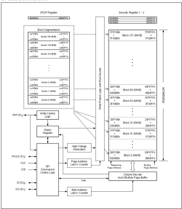
Figure 2. W25Q64JW Serial Flash Memory Block Diagram
