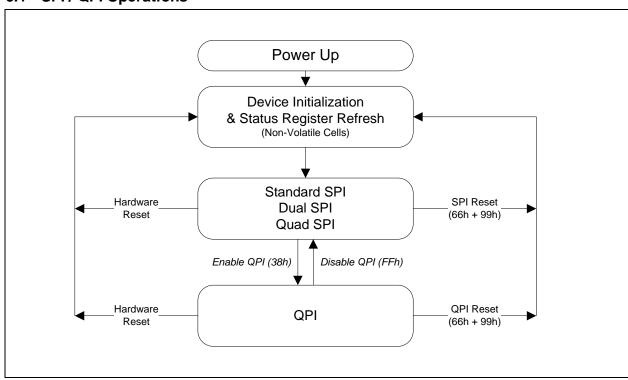
Figure 3. W25Q64JW Serial Flash Memory Operation Diagram
