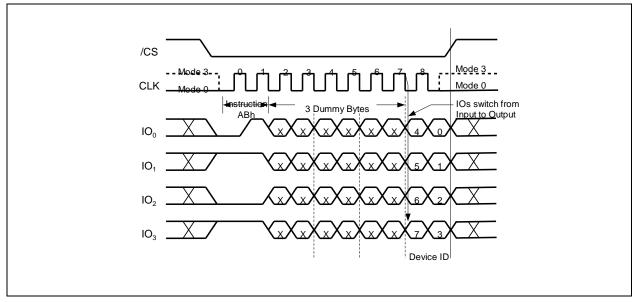
Figure 38d. Device ID Instruction (QPI Mode)
