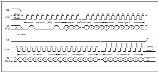
Figure 46. Program Security Registers Instruction (SPI Mode only)
