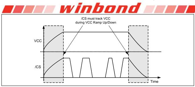
Figure 58b. Power-up, Power-Down Requirement
