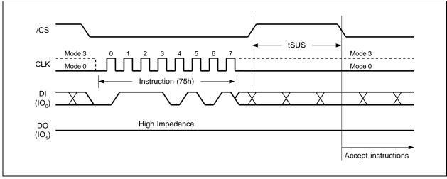
Figure 35a. Erase/Program Suspend Instruction (SPI Mode)
