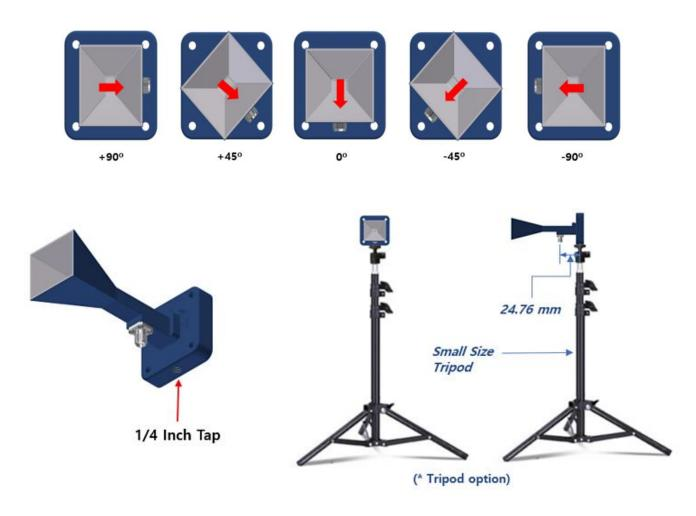
\*\* Depending on the size of the tripod, installation may not be possible. Please check the drawing dimensions.
