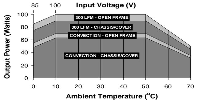
**Derating requirements** – Chart above applies to models 1003 thru 1008 only. 100W 300 LFM forced air, open frame. 70W convection cooled open frame. Derate 10% with Chassis and Cover. Derate 1.0W<sub>OUT</sub> / 1V<sub>IN</sub> below 100V<sub>IN</sub> and between 100V<sub>IN</sub> and 85V<sub>IN</sub>. Use larger of the two deratings when using chassis/cover below 100V<sub>IN</sub>. Derate output power linearly to 50% between 50° and 70°C.
