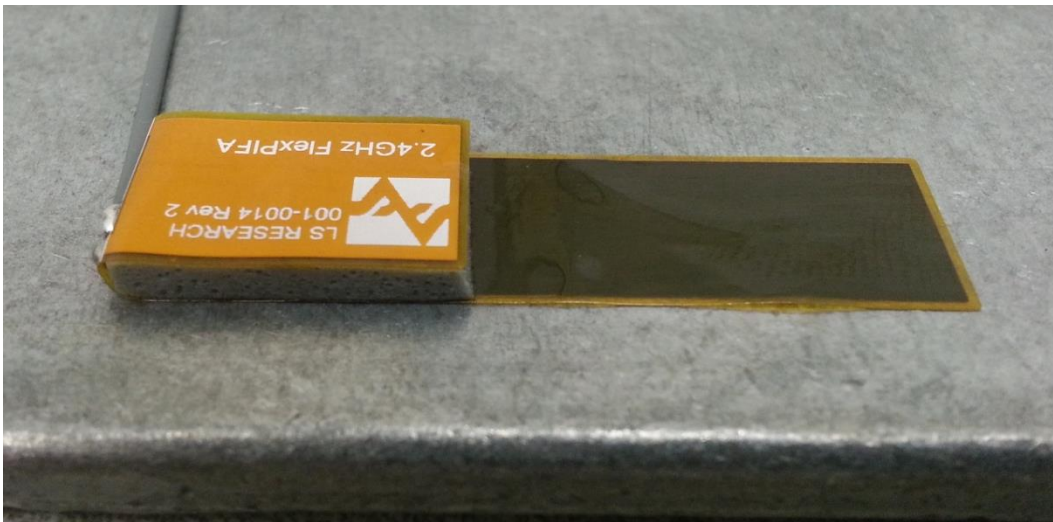
Figure 24 FlexPIFA Mounted on Metal
