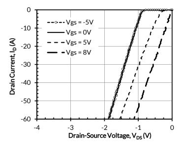
Figure 9. 3rd quadrant characteristics at  $T_J = -55$ °C
