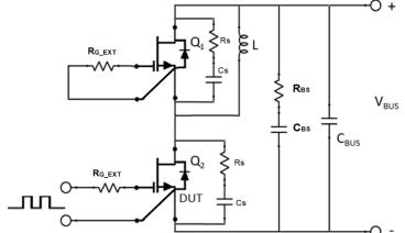
Figure 23. Schematic of the half-bridge mode switching test circuit. Note, a bus RC snubber ( $R_{BS}$  = 2.5 $\Omega$ ,  $C_{BS}$ =100nF) is used to reduce the power loop high frequency oscillations.
