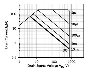
Figure 17. Safe operation area at  $T_C = 25$ °C, D = 0, Parameter t<sub>n</sub>
