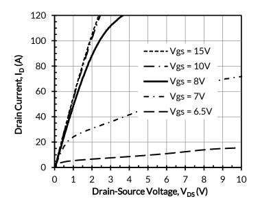
120 100 Drain Current, I<sub>D</sub> (A) 80 60 Vgs = 15V Vgs = 8V 40 Vgs = 7V- Vgs = 6.5V 20 Vgs = 6V 0 1 2 3 5 10 Drain-Source Voltage,  $V_{DS}(V)$
