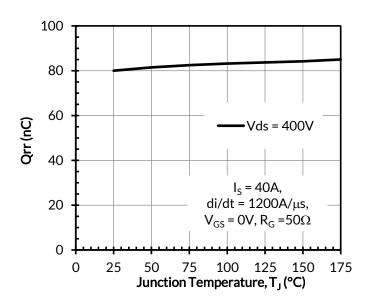
Figure 18. Reverse recovery charge Qrr vs. junction temperature
