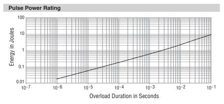
The energy absorbed by the resistor expressed in Joules can be calculated by multiplying the peak power of the pulse in watts times the length of the pulse in seconds.
