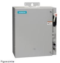
Pump control panel, Size 2 1/2, Three phase full voltage, Solid-state overload relay, OLR amp range 25-100A, 190-220/220-240V 50/60Hz coil, Standard type contactor, 100A circuit breaker, HOA Sel Sw. <(>&<)> Start P.B., Enclosure NEMA type 3/3R, Weather proof outdoor use
