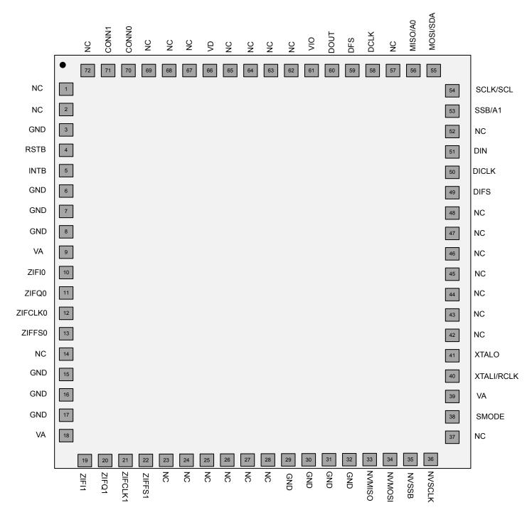
Figure 1.1. Si4692 Pinout Diagram
