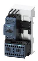
FUSELESS LOAD FEEDER REVERSING OPERATION, AC 400V, S00 1.4. . .2A, AC 110/120V 50/60HZ SCREW TERMINAL FOR BUSBAR SYSTEMS 60MM TYPE OF ASSIGNMENT 2,IQ = 150KA (ALSO FULFILLS TYPE OF ASSIGNMENT 1) 1NC (CONTACTOR)
