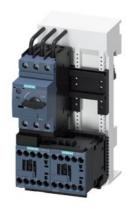
Fuseless motor starter Reversing operation 600VAC Size S00 0.11-0.16a 24V DC screw connection For snapping onto 60 mm busbar systems Type of coordination 2 IQ = 150 KA Also full fills type Of coordination 1 1NC (per contactor)
