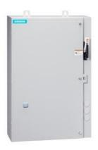
Non-reversing motor starter, Size 1, Three phase full voltage, Solid-state overload relay, OLR amp range 10-40A, Combination type, 60A fusible disconnect, 60A/250V fuse clip, Encl NEMA type 4X 304 S-Steel, Water/dust tight noncorrosive, Extra-wide enclosure
