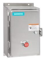
Non-reversing motor starter, Size 1, Three phase full voltage, Solid-state overload relay, OLR amp range 5.5-22A, Non-combination type, Encl. type 4X 304 S. Steel, Water/dust tight noncorrosive, Standard width enclosure
