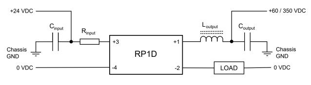
$C_{input}$  = 1 nF 2 kV (Y2 class, ceramic disc)  $R_{input}$  = 10  $\Omega$  (0.25 W) L<sub>output</sub> = ferrite core + 4 turns C<sub>output</sub> = 1 nF 2 kV (Y2 class, ceramic disc)
