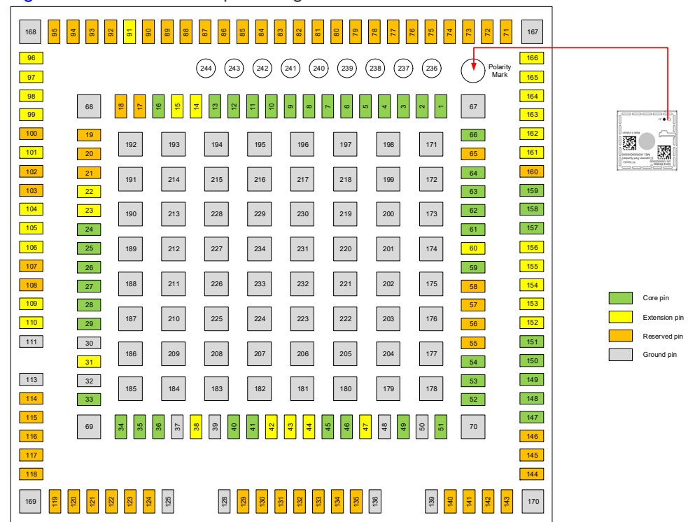
Figure 10-1: Pin Configuration (Top View, Through Module)
