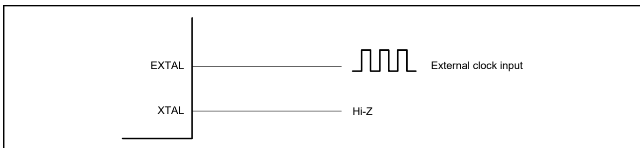
Figure 9.5 Equivalent circuit for external clock
