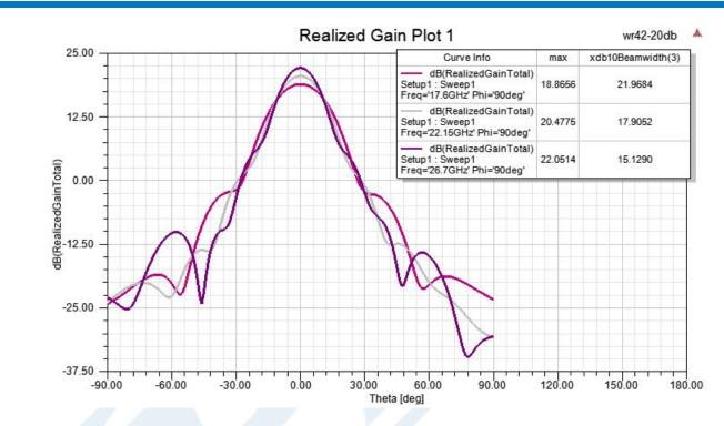
WR-42 Standard Gain Horn with 20 dBi gain, End Launch 2.92mm Female connector from Pasternack Enterprises has same day shipment for domestic and International orders. Our RF, microwave and millimeter wave products maintain a 99.4% availability and are part of the broadest selection in the industry.
