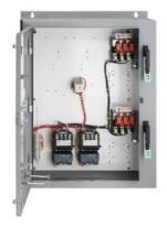
Duplex starter with alternator Size 2.5 Three phase full voltage Solid-state overload relay OLR amp range 25-100A 110VAC 50Hz / 120VAC 60Hz Coil Combination type Two 100A disconnect switches Encl NEMA type 4 painted steel Water/dust tight weather proof
