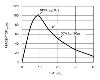
Fig.7 ESD pulse waveform per IEC61000-4-2
