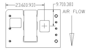
Figure 16. T<sub>ref</sub> Temperature Measurement Location.
