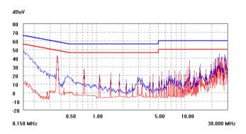
$\label{eq:Figure 18.} \textbf{EMC signature using above filter, KHHD006A0A}.$
