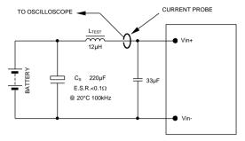
NOTE: Measure input reflected ripple current with a simulated source inductance (L<sub>TEST</sub>) of 12µH. Capacitor C<sub>S</sub> offsets possible battery impedance. Measure current as shown
