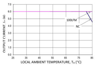
Figure 15. Output Current Derating for the Open Frame KHHD006A0A in the Transverse Orientation; Airflow Direction from Vin(+) to Vin(-); Vin = 48V.
