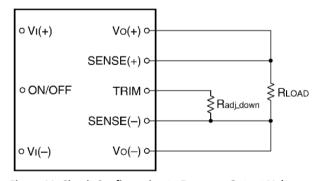
Figure 11. Circuit Configuration to Decrease Output Voltage.
