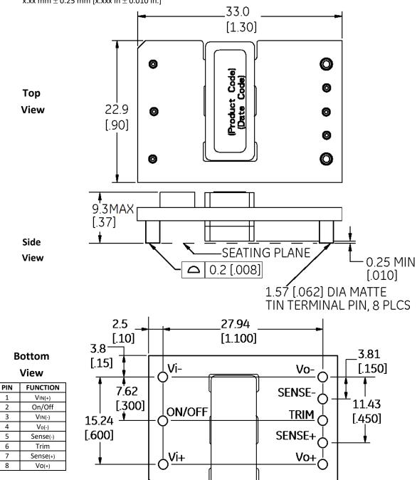
18-75Vdc Input; 5.0Vdc, 6A Output
