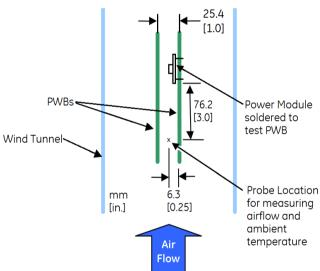
Figure 13. Thermal Test Setup.
