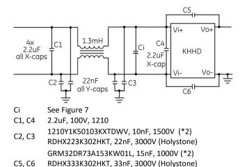
Figure 17. Suggested Configuration for EN55032 Class B.
