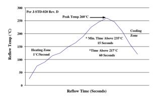
Figure 22. Recommended linear reflow profile using Sn/Ag/Cu solder.
