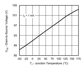
**Drain Source Breakdown vs. Junction Temperature**
