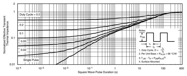
Normalized Thermal Transient Impedance, Junction-to-Ambient
