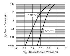
**Source Drain Diode Forward Voltage**
