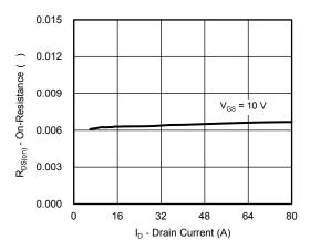
On-Resistance vs. Drain Current
