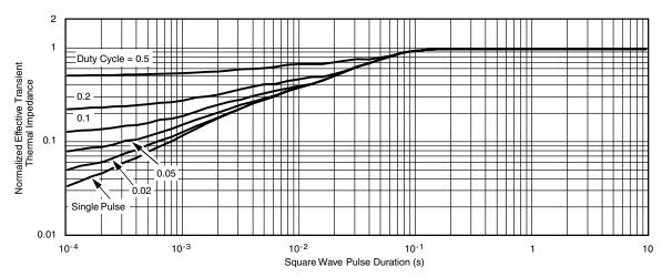
Normalized Thermal Transient Impedance, Junction-to-Case
