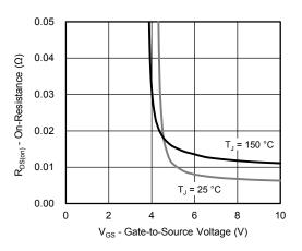
On-Resistance vs. Gate-to Source Voltage
