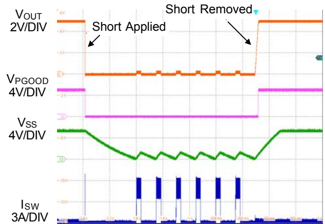
Figure 3. Short-Circuit Protection and Recovery
