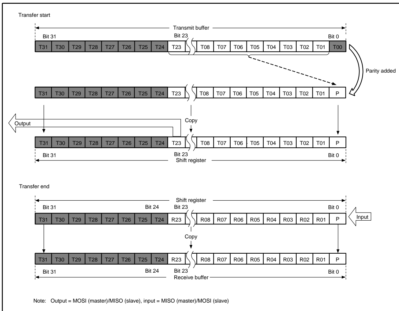
Figure 44.19 MSB First Transfer (24-Bit Data, Parity Enabled)
