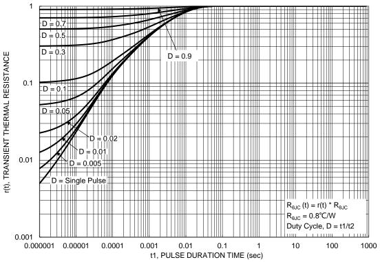
Figure 13. Transient Thermal Resistance
