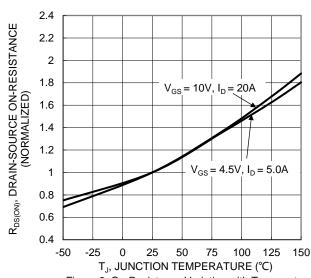
Figure 6. On-Resistance Variation with Temperature
