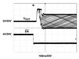
FIGURE 21. EL5378 ENABLED RESPONSE
