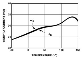
FIGURE 26. ± SUPPLY CURRENT vs TEMPERATURE
