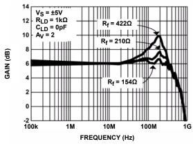
FIGURE 6. EL5378 FREQUENCY RESPONSE FOR VARIOUS  $R_{\rm F}$
