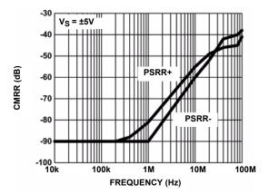
FIGURE 12. DIFFERENTIAL PSRR vs FREQUENCY
