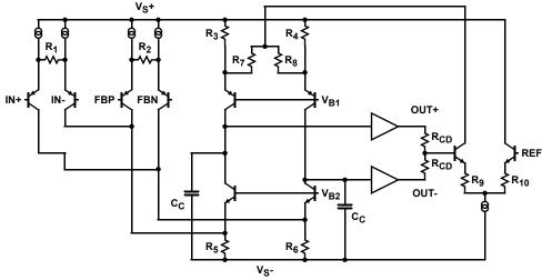
FIGURE 34. SIMPLIFIED SCHEMATIC
