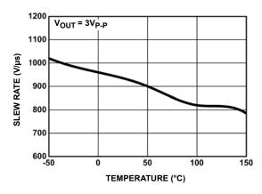
FIGURE 29. SLEW RATE vs TEMPERATURE
