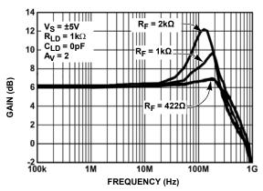
FIGURE 1. EL5178 FREQUENCY RESPONSE FOR VARIOUS RF
