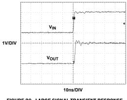
FIGURE 20. LARGE SIGNAL TRANSIENT RESPONSE
