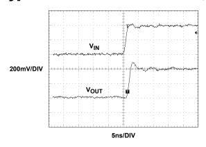
FIGURE 19. SMALL SIGNAL TRANSIENT RESPONSE
