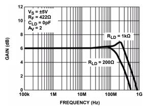
FIGURE 4. EL5178 FREQUENCY RESPONSE FOR VARIOUS R<sub>LD</sub>
