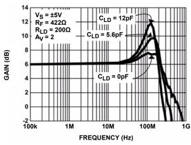
FIGURE 8. EL5378 FREQUENCY RESPONSE FOR VARIOUS CLD
