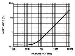
FIGURE 13. OUTPUT IMPEDANCE vs FREQUENCY
