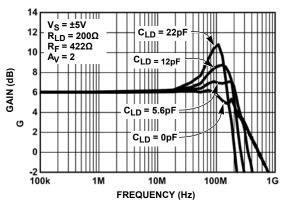
FIGURE 3. EL5178 FREQUENCY RESPONSE FOR VARIOUS  $C_{LD}$
