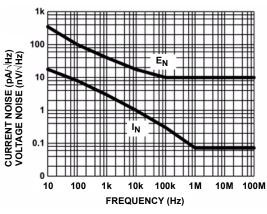
FIGURE 10. VOLTAGE AND CURRENT NOISE vs FREQUENCY
