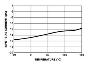
FIGURE 28. INPUT BIAS CURRENT vs TEMPERATURE
