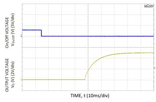
Figure 5. Typical Start-up Using Remote On/Off, negative logic version shown ( $V_{IN} = 48V$ ,  $I_0 = I_{0,max}$ ).
