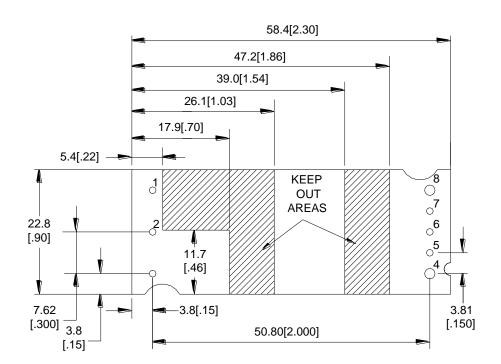
TH Recommended Pad Layout (Component Side View)
