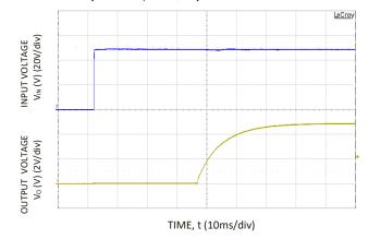
Figure 6. Typical Start-up Using Input Voltage ( $V_{IN}$  = 48V,  $I_0$  =  $I_{O,max}$ ).
