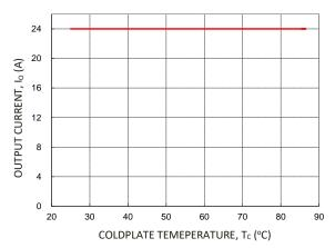
Figure 22. Derated Output Current versus Cold Wall Temperature with local ambient temperature around module at 85C;  $V_{\rm IN}$  =24V or 48V.
