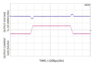
Figure 3. Transient Response to 0.1A/µS Dynamic Load Change from 50% to 75% to 50% of full load, Vin=24V
