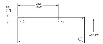
Figure 14.  $T_{\text{ref}}$  Temperature Measurement Location for Module with Heat plate.
