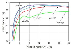
Figure 1. Converter Efficiency versus Output Current.
