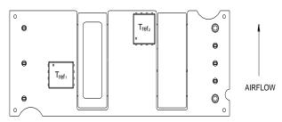
Figure 13.  $T_{\text{ref}}$  Temperature Measurement Locations for Open Frame Module.
