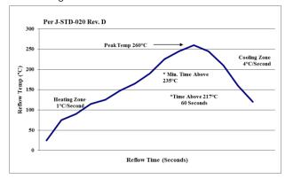
Figure 26. Recommended linear reflow profile using Sn/Ag/Cu solder.
