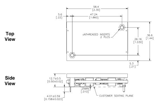
${}^\star \text{For optional pin lengths},$  see Table 2, Device Coding Scheme and Options
