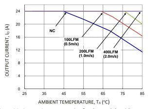
Figure 20. Output Current Derating for the Module with - 18 Heatplate; Airflow in the Transverse Direction from  $V_{out}(-)$  to  $V_{out}(+)$ ;  $V_{IN} = 24V$ ,  $V_{O} = 5V$ .
