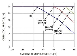
Figure 17. Output Current Derating for the Module with 18H Heatplate; Airflow in the Transverse Direction from  $V_{out}(-)$  to  $V_{out}(+)$ ;  $V_{IN}$  =48V,  $V_{O}$ =5V
