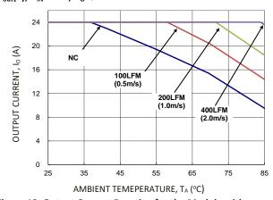
Figure 19. Output Current Derating for the Module with Heatplate; Airflow in the Transverse Direction from  $V_{out}(-)$  to  $V_{out}(+)$ ;  $V_{IN}=24V$ ,  $V_0=5V$ .
