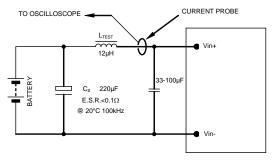
NOTE: Measure input reflected ripple current with a simulated source inductance ( $L_{\text{TST}}$ ) of 12µH. Capacitor  $C_{\text{S}}$  offsets possible battery impedance. Measure current as shown above.
