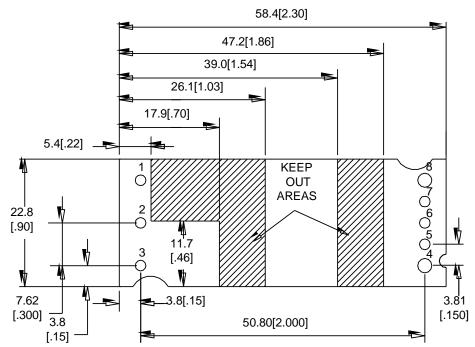
SMT Recommended Pad Layout (Component Side View)
