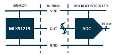
Figure 4: Schematic of ratiometric mode
