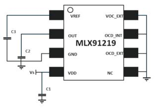
Figure 12: Application Diagram for SOIC8 package, bidirectional OCD<sub>EXT</sub>.
