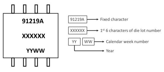
Figure 22. SOIC8 package marking
