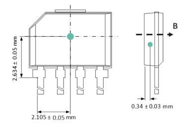
Figure 14: VA/SIL-4L Magnetic center and sensor's active measurement direction B
