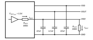
Figure 13: Case when the external resistance on reference pin is low.
