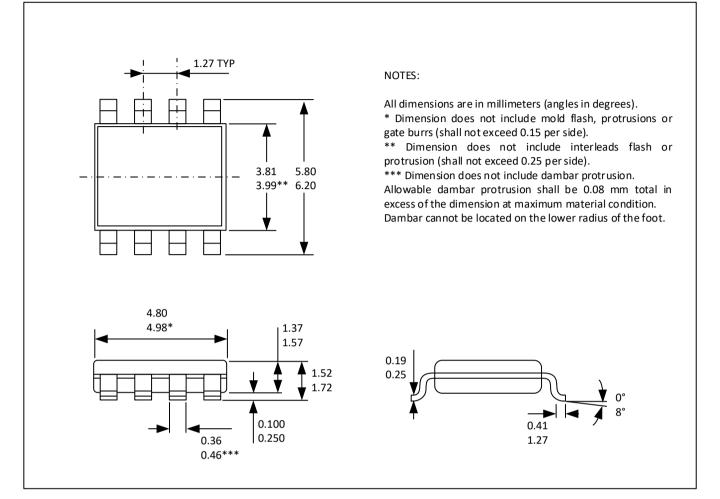
Figure 23: SOIC8 package
