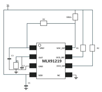
Figure 11: Application Diagram for SOIC8 package, unidirectional OCD<sub>EXT</sub>.
