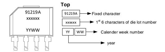
Figure 15. VA/SIP 4L (single in-line package) / 18mm lead length - Package Information
