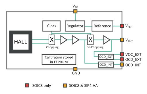
Figure 3: Block Diagram of the MLX91219.
