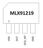
Figure 6: Pinout of SIP4-VA package.
