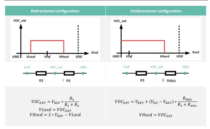
Table 19: External OCD, bidirectional and unidirectional configurations
