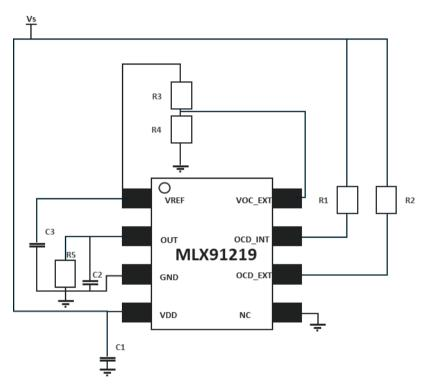
Figure 10: Application Diagram for SOIC8 package, bidirectional OCD<sub>EXT</sub>.
