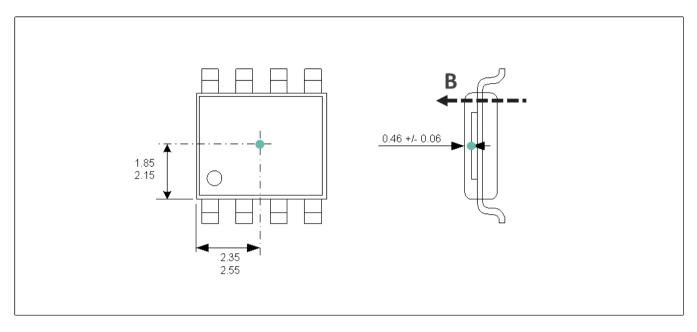
Figure 21: VA/SIL-4L Magnetic center and sensor's active measurement direction B
