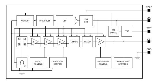
Figure 3: Block Diagram of the MLX91217:
