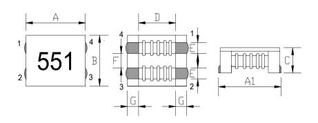
A: 15.0±0.5 mm A1:15.0±0.6 mm B: 13.0±0.4 mm C: 6.0 Max.  $\mathbf{m}\mathbf{m}$ D: 9.0 Typ. mm E: 2.7±0.2 mm F: 3.8±0.2 mm G: 3.0±0.2 mm
