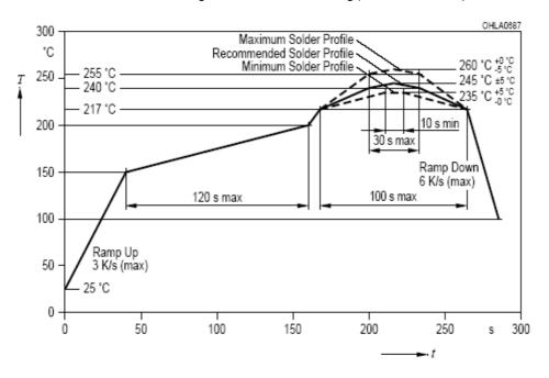
IR-Reflow Soldering Profile for lead free soldering (Acc. to J-STD-020B)
