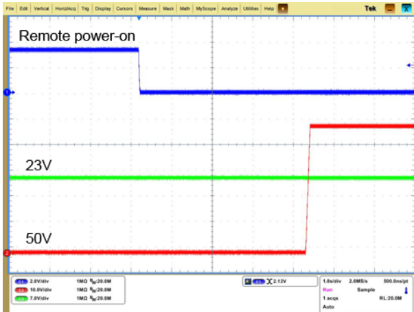
Remote power-on ( V_{in} = 48\text{ V} , V_{out1} = 50\text{ V} , V_{out2} = 23\text{ V} )
