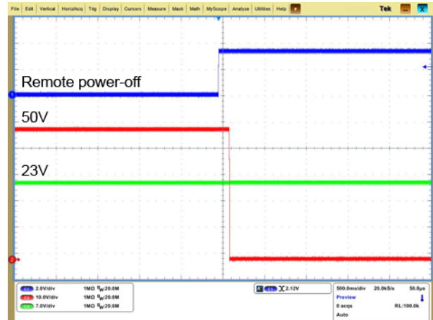
Remote power-off ( V_{in} = 48\text{ V} , V_{out1} = 50\text{ V} , V_{out2} = 23\text{ V} )
