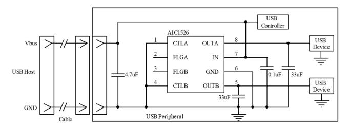
Fig. 12 Inrush Current-Limit Application
