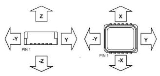
Figure 3. Accelerometer measuring directions
