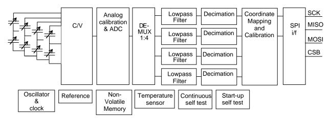
Figure 1. SCA3100-D07 Block diagram
