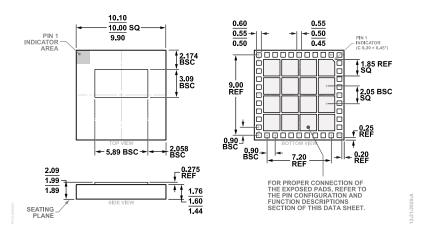
Figure 27. 40-Terminal Land Grid Array Package [LGA] 10 mm × 10 mm Body and 1.99 mm Package Height (CC-40-10) Dimensions shown in millimeters
