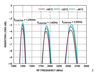
Figure 7. Insertion Loss vs. RF Frequency for Nominal 9% Bandwidth at Various Temperatures and Center Frequencies
