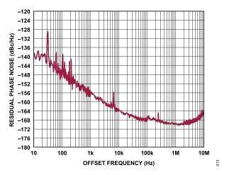
Figure 17. Residual Phase Noise vs. Offset Frequency for  $f_{CENTER}$ = 1.9 GHz
