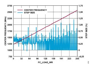
Figure 16. Center Frequency and Step Size vs. FC\_LOAD\_WR
