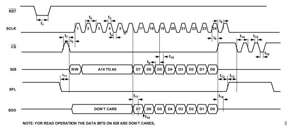
Figure 2. Timing Diagram
