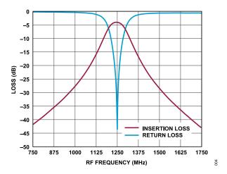
Figure 5. Insertion Loss and Return Loss vs. RF Frequency for Nominal 9% Bandwidth at 1.25 GHz
