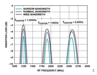
Figure 11. Insertion Loss vs. RF Frequency at Various Bandwidths and Center Frequencies
