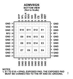
Figure 3. Pin Configuration
