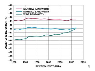
Figure 10. Percentage Away from f<sub>CENTER</sub> for Lower 20 dB Rejection vs. RF Frequency for Various Bandwidths
