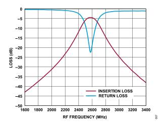
Figure 8. Insertion Loss and Return Loss vs. RF Frequency for Nominal 9% Bandwidth at 2.6 GHz
