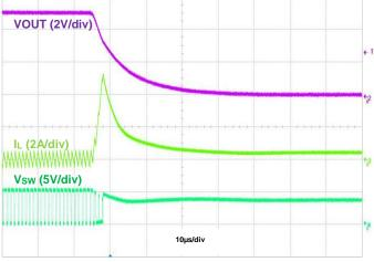
Figure 12. Output Short Protection, IOUT = 0A
