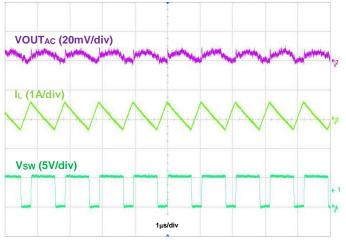
Figure 48. Output Voltage Ripple, VOUT = 5.2V, IOUT = 50mA
