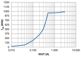
Figure 19. fsw vs. Load
