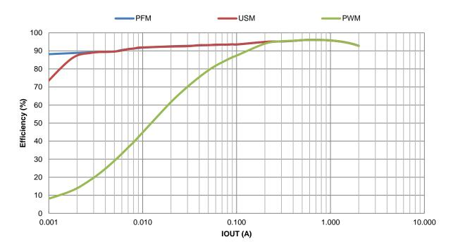
Figure 2. Efficiency vs. Output Current, VIN = 3.6V, VOUT = 5.2V, L = 1 $\mu$ H
