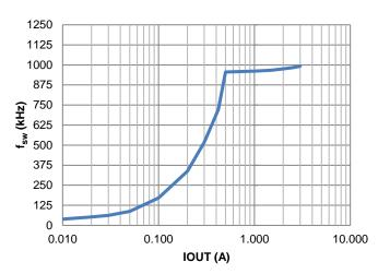
Figure 33. f<sub>SW</sub> vs. Load
