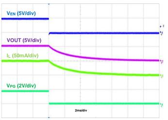
Figure 11. Shutdown Using EN, IOUT = 50mA
