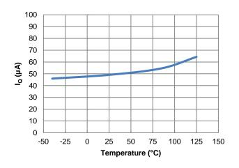
Figure 18. Iq vs. Temperature,  $V_{EN}$  = VIN,  $V_{MODE}$  = GND, R1 = 1.05M $\Omega$ , R2 = 200k $\Omega$
