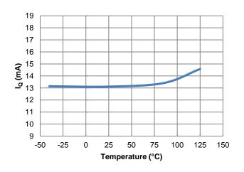
Figure 45. IQ vs. Temperature,  $V_{EN} = V_{MODE} = VIN, R1 = 1.05 M\Omega, R2 = 200 k\Omega$
