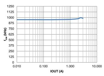
Figure 47. fsw vs. Load
