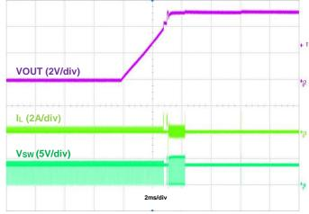
Figure 13. Output Short Recovery, IOUT = 0A
