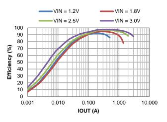
Figure 42. Efficiency vs. Output Current, VOUT = 3.3V
