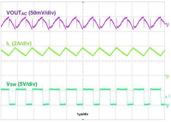
Figure 35. Output Voltage Ripple, VOUT = 5.2V, IOUT = 2A
