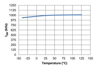
Figure 46. fsw vs. Temperature, IOUT = 0A
