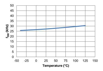
Figure 32. fsw vs. Temperature, IOUT = 0A
