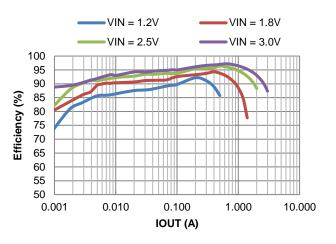
Figure 28. Efficiency vs. Output Current, VOUT = 3.3V
