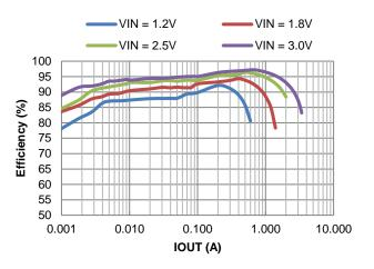
Figure 15. Efficiency vs. Output Current, VOUT = 3.3V
