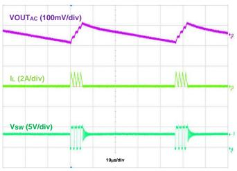
Figure 34. Output Voltage Ripple, VOUT = 5.2V, IOUT = 50mA
