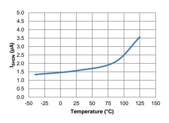
Figure 8. I<sub>SHDN</sub> vs. Temperature
