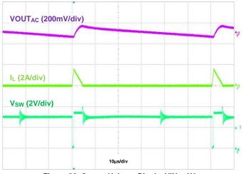
Figure 36. Output Voltage Ripple, VIN = 3V, VOUT = 3.3V, IOUT = 50mA
