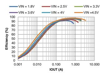
Figure 41. Efficiency vs. Output Current, VOUT = 5.2V
