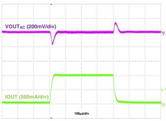
Figure 52. Load Transient, IOUT = 50mA to 1A to 50mA
