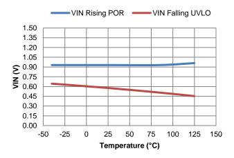
Figure 9. VIN Power-On Reset and UVLO vs. Temperature
