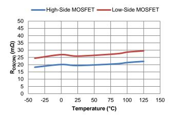
Figure 5. Power MOSFET RDS(ON) vs. Temperature
