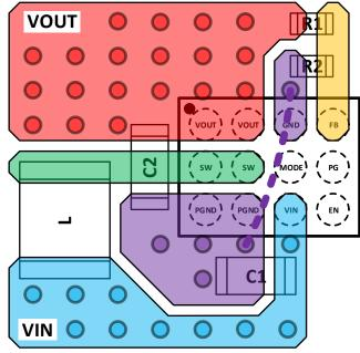
Figure 56. Recommended PCB Layout
