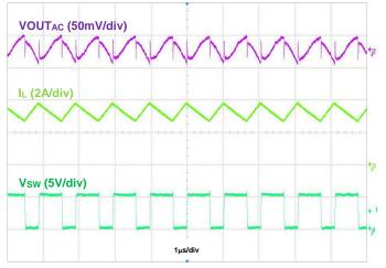
Figure 20. Output Voltage Ripple, VOUT = 5.2V, IOUT = 50mA
