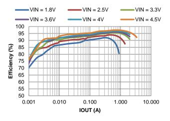
Figure 27. Efficiency vs. Output Current, VOUT = 5.2V
