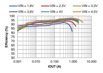
Figure 14. Efficiency vs. Output Current, VOUT = 5.2V
