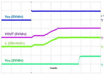
Figure 10. Startup Using EN, IOUT = 50mA
