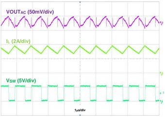
Figure 49. Output Voltage Ripple, VOUT = 5.2V, IOUT = 2A
