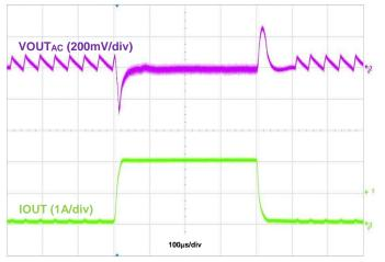
Figure 40. Load Transient, IOUT = 50mA to 2A to 50mA
