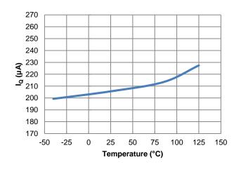
Figure 31. IQ vs. Temperature,  $V_{EN}$  = VIN,  $V_{MODE}$  = Floating, R1 = 1.05M $\Omega$ , R2 = 200k $\Omega$
