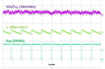
Figure 50. Output Voltage Ripple, VIN = 3V, VOUT = 3.3V, IOUT = 50mA
