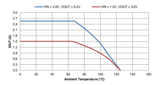
Figure 55. Output Current Derating Curve vs. Ambient Temperature
