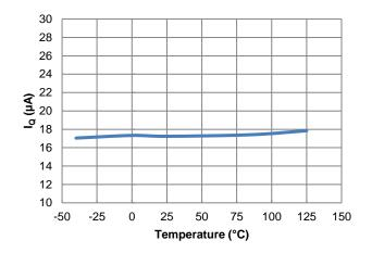
Figure 7. IQ vs. Temperature, VEN = VIN, VFB = 1.0V
