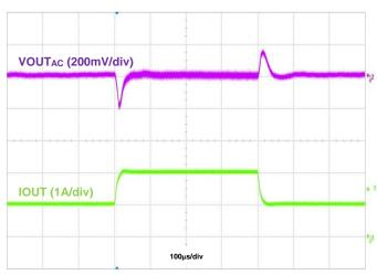
Figure 53. Load Transient, IOUT = 1A to 2A to 1A
