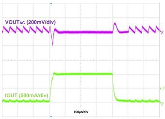
Figure 24. Load Transient, IOUT = 50mA to 1A to 50mA
