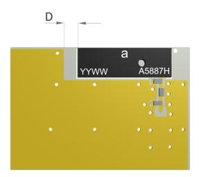
Additional ground and components near the antenna should be at a distance of at least 2mm. Where possible the antenna should be clear of ground from both sides, although the antenna can work well with a minimum clearance of  $D \ge 2$  mm as shown in the drawing above.
