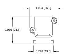
P/N **955-50-SR-8-10** CABLE RANGE = 0.315 - 0.394 P/N **955-50-SR-11-14** CABLE RANGE = 0.433 - 0.551 P/N **955-50-SR-14-16** CABLE RANGE = 0.551 - 0.630
