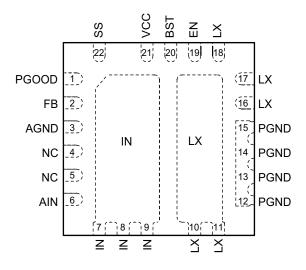
22-Pin 4mm x 4mm QFN (Top View)
