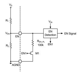
Figure 2. Enable Internal Circuit
