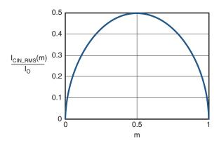
Figure 7. I<sub>CIN</sub> vs. Voltage Conversion Ratio
