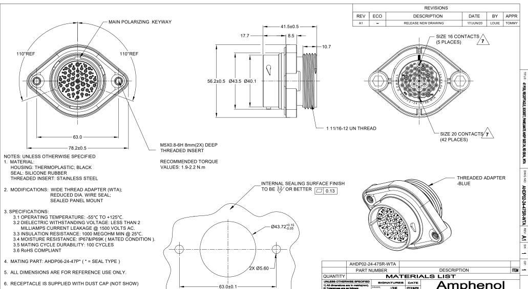
CONTACT MIN. INSUL MAX. INSUL TYPICAL WIRE CURRENT SIZE O.D. O.D. RANGE RATING 1.02 mm 2.10 mm 16-22 AWG 7.5 AMPS 20 (.040 in) (.083 in) (1.5-0.35mm<sup>2</sup>) 1.35 mm 2.62 mm 14-20 AWG 13 AMPS 16 (.053 in) (.103 in) (2.0-0.5mm<sup>2</sup>)
