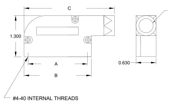
(162-000-925R000) 0.185" 0.248" 0.290" 0.324" MAX CABLE Ø WITHOUT GROMMETS 0.393" 981-YYY-030R121 **SERIES POSITIONS** 009 015 025 **MATERIAL** 030 = ZINC COLOR 12 = NICKEL OVER COPPER
