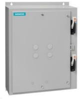
Duplex starter w/o alternator, Size 1 3/4, Three phase full voltage, Solid-state overload relay, OLR amp range 10-40A, 110V 50Hz / 120V 60Hz coil, Combination type, Two 40A circuit breakers, Enclosure NEMA type 12, Dust/drip proof for indoors
