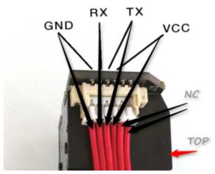
If your sensor has all the same-color wires, The first wire from the left is ground, then the two data pins, then power. You'll have to cut, strip and solder the wires.
