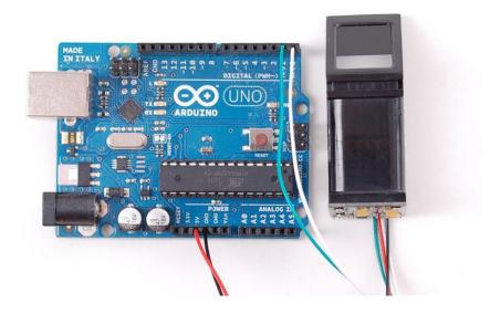
Start up the SFGDemo software and click Open Device from the bottom left corner. Select the COM port used by the Arduino.
