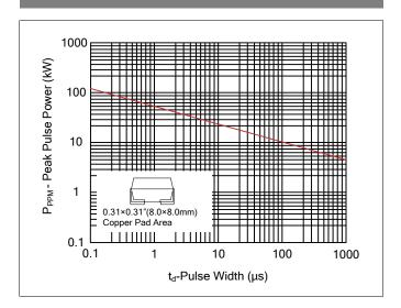
Figure 2. Pulse Derating Curve
