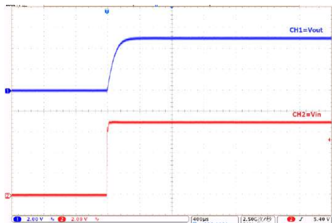
Power-Up at V_{OUT}=5.0V : (I_{OUT}=150mA)
