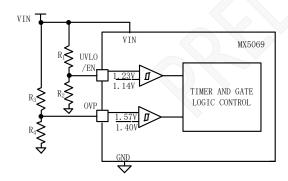
The four resistor values are calculated as follows:
