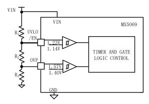
The undervoltage lockout (UVLO) and overvoltage trip point are adjusted using an external voltage divider network of R1,
