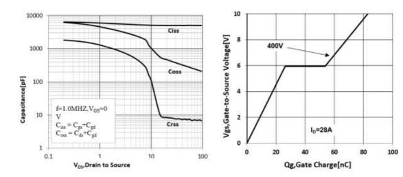
Figure 12 Typical Capacitance vs Drain to Source Voltage
