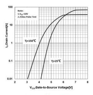
Figure 6 Typical Transfer Characteristics
