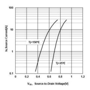
Figure 7 Typical Body Diode Transfer Characteristics
