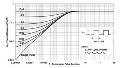
Figure 5 Maximum Effective Thermal Impedance, Junction to Case
