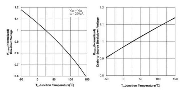
Figure 10 Typical Theshold Voltage vs Junction Temperature
