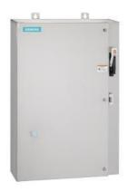
Non-reversing motor starter, Size 4, Three phase full voltage, Solid-state overload relay, OLR amp range 50-200A, Combination type, 200A non-fusible disconnect, Encl NEMA type 4X 304 S-Steel, Water/dust tight noncorrosive, Standard width enclosure
