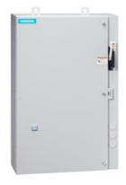
Non-reversing motor starter, Size 2 1/2, Three phase full voltage, Solid-state overload relay, OLR amp range 25-100A, 110V 50Hz / 120V 60Hz coil, Combination type, 100A fusible disconnect, 100A/250V fuse clip, Encl NEMA type 4X 304 S-Steel, Water/dust tight noncorrosive, Standard width enclosure
