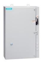
Non-reversing motor starter, Size 1, Three phase full voltage, Solid-state overload relay, OLR amp range 0.25-1A, Combination type, 30A non-fusible disconnect, Encl NEMA type 4X 304 S-Steel, Water/dust tight noncorrosive, Extra-wide enclosure
